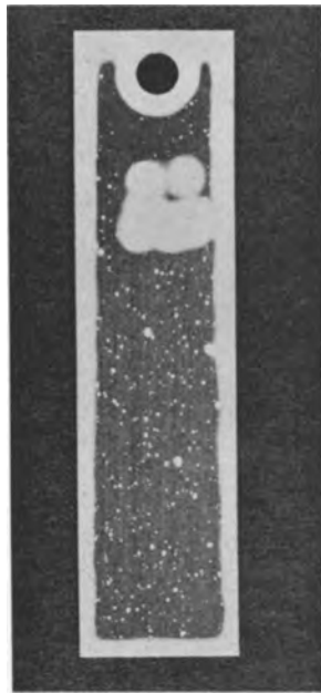
Fig. 4. Specimen of Zircaloy-2 oxidized for 50 hr at 600°C in 25 mm oxygen. Note the effect of specimen geometry on the oxidation rate. White areas have undergone transition. Magnification approximately 1¼X.
