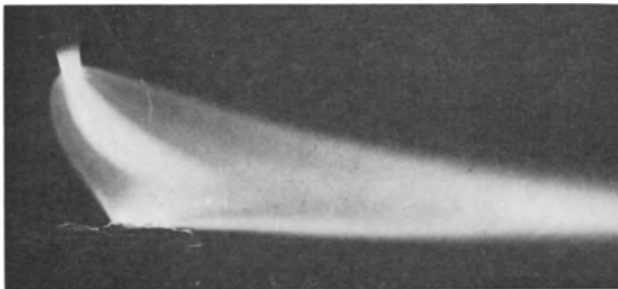
Fig. 3. High intensity arc tail flame in argon: anode: graphite crucible containing metallic aluminum; cathode, \frac{3}{8} in. diameter, graphite.
