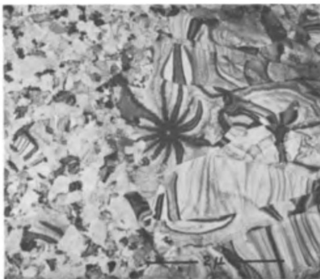
Fig. 2. Electron micrograph showing crystalline regions of widely different grain size, beam-crystallized; anodic tantalum oxide film 250Å thick.
