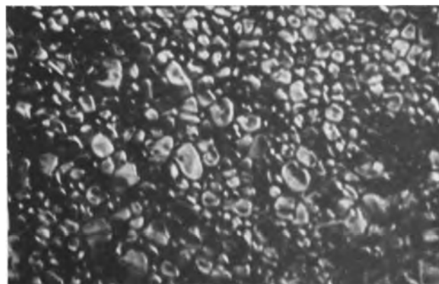
Fig. 4. Same as Fig. 3. except the annealing temperature was very close to, or at, the incipient fusion point. Magnification 520X.
