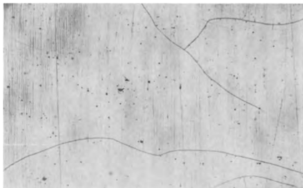
Fig. 6. Type Y cracking in chromium plated on nickel polished on canvas lap using Buehler No. 1 alumina. Magnification approximately 100X.
