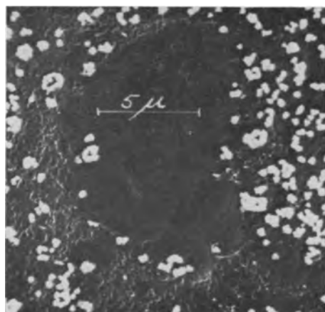
Fig. 2. Electron micrograph of As-Te-I glass (20 a/o I), polished and etched surface, two-step replica technique.
