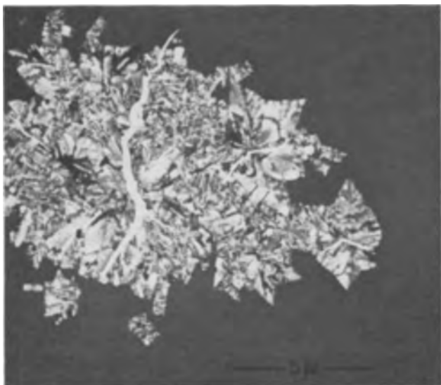
Fig. 3. Electron micrograph of crystallized region in thick anodic film, beam-crystallized; anodic tantalum oxide film 1000Å thick.
