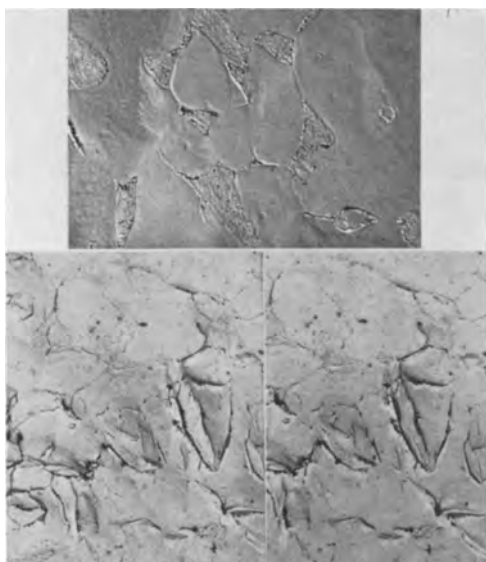
Fig. 9. Structure of hot-rolled plus cold-rolled alloy, corroded 100 days in 360°C water. a (upper), Alloy substrate, 6000X. b (lower), stereo pair of oxide film surface (negative replicas). Magnification approximately 3000X.
