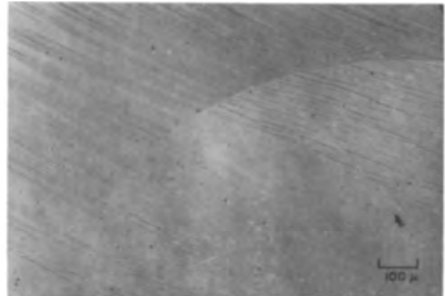
Fig. 5. Features characteristic of a facet and of a curved interface during growth of an InSb crystal. Magnification X150.
