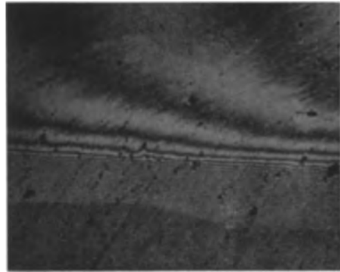
Fig. 3. Differentiated N-P junction of GaAs formed by selenium diffusion at 1050°C, 120 hr. (Wafer surface at left had 20,000Å SiO, wafer surface at right had only 2500Å SiO.) Magnification approximately 150X (reduced to approximately 110X).
