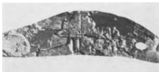
Fig. 4. Specimen of zone-refined iron after 48 hr in 44.4% \text{NH}_4\text{NO}_3 , 5.9% \text{NH}_3 solution, 25°C, showing unequal attack of grains.
