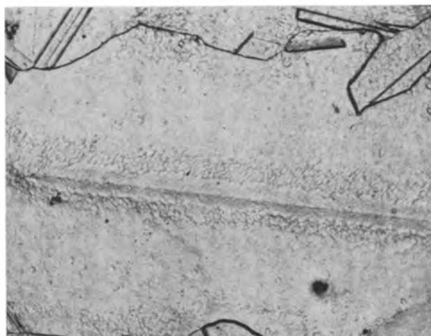
Fig. 7. Same as Fig. 6 except it is about 6-7 mm away from the border of molten zone. Magnification 37X.
