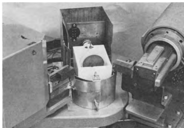
Fig. 2. Cell mounted on spectrogoniometer. Electrical wiring and part of the shielding were removed for this photograph.
