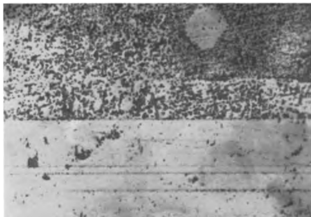
Fig. 6. Photomicrograph of cross section through SiC crystal showing junction produced by nitrogen doping during growth; electrolytically etched in HF solution. Magnification 250X.
