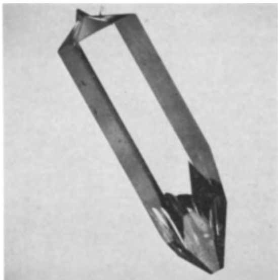
Fig. 3. A synthetically grown beryllium oxide crystal (dihexagonal hemimorphic class). The habit is apparent: hexagonal prism elongated along the c -axis. The presence of the hemipyramid indicates the lack of a center of symmetry. The small hemipyramid at the center of the large negative basal complex is the visible portion of another crystal having reversed polarity but in optical continuity with the crystal surrounding it (25X).
