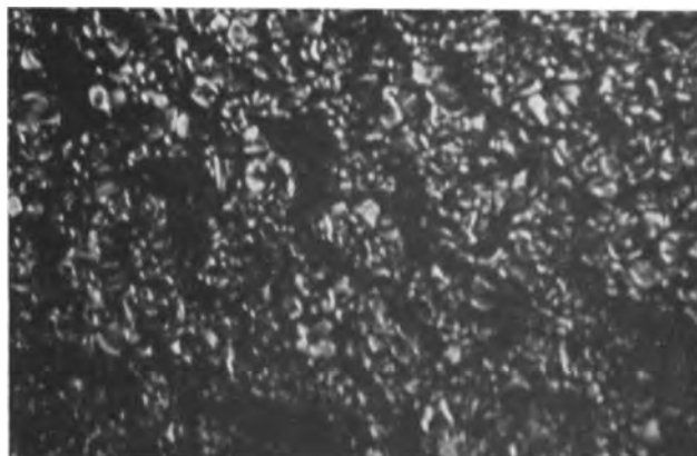
Fig. 3. Polycrystalline silicon film annealed 30 min at about 5^\circ\text{-}10^\circ\text{C} below the melting point of silicon. Magnification 520X.
