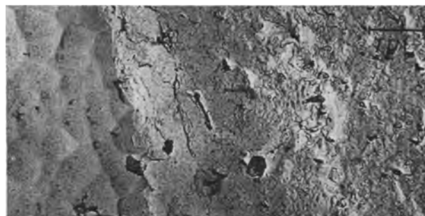
Fig. 7. Surface of cuprous oxide, partially covered with cupric oxide (right side); T = 300^\circ\text{C} ; p_{\text{O}_2} = 15.8 mm Hg.
