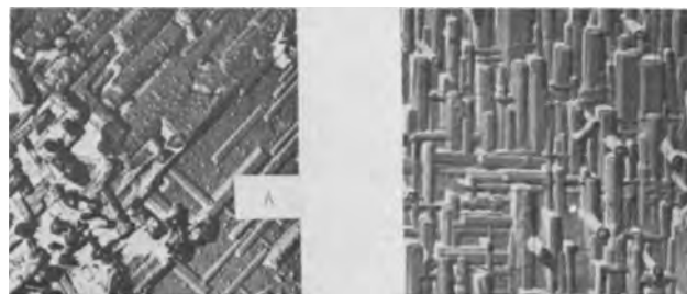
Fig. 2. Typical electron micrographs of alloy, FeSn 2 , formed on a polycrystalline substrate. Tin electrodeposited from a phenolsulfonic acid electrolyte. Magnification 17,000X before reduction for publication.
