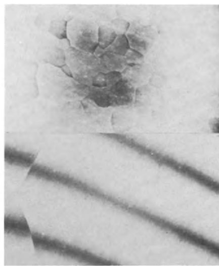
Fig. 4. Surface of a prepared 60-40 Pt-Rh substrate after heating to deposition temperature. (a) (top) Interference contrast micrograph. Magnification 35X; (b) (bottom) interferogram of grain boundary. Magnification 225X.
