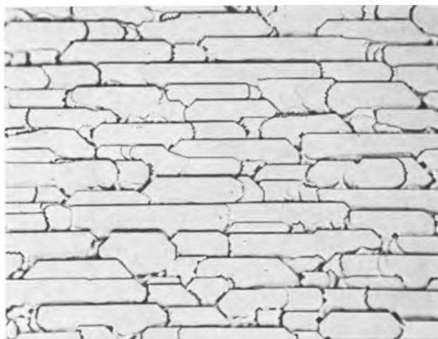
Fig. 1. Layer growth structure on a copper single crystal with a surface near (100). Typical deposition conditions: 20 ma/cm 2 , 30 min, from a N CuSO 4 + N H 2 SO 4 solution at 35°C. X435.
