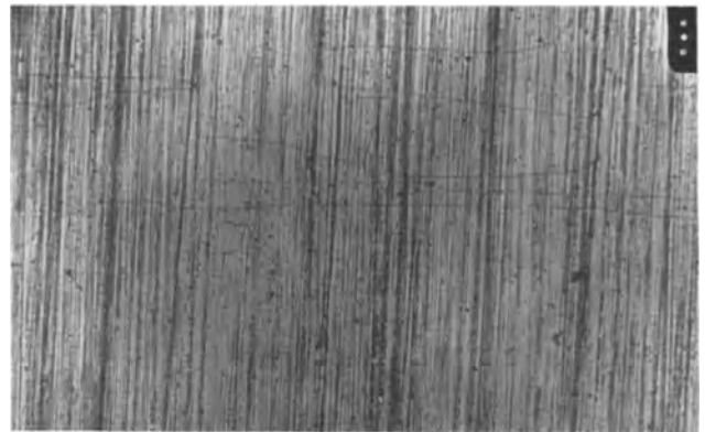
Fig. 5. Type Y cracking in chromium plated on nickel polished on 400-grit silicon carbide paper. Magnification approximately 100X.
