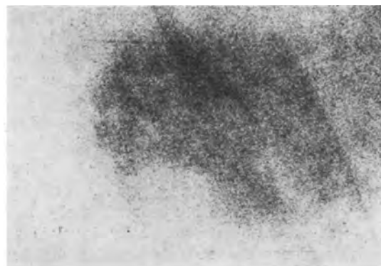
Fig. 3. A Berg-Barrett image of an electrodeposit formed at 15^\circ\text{C} on the substrate shown in Fig. 2. X15.
